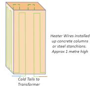
Thermatek stanchion heaters can be installed against concrete columns or around steel stanchions within the cold room.
